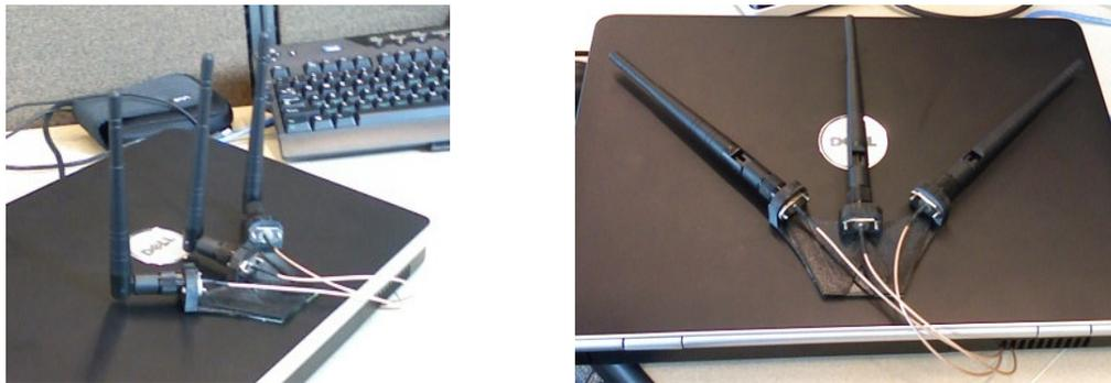
**Figure 5.3:** One of the three laptops, pictured here, includes a custom antenna mount for a 2.4 GHz linear array.
