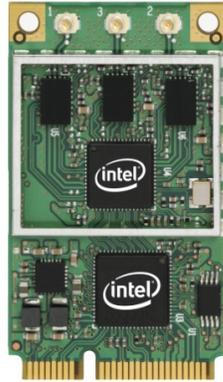
**Figure 5.4: The Intel Wireless Wi-Fi Link 5300. This 802.11n device has three transmit/receive antennas, operates on both 2.4 GHz and 5 GHz frequency bands, and supports up to three spatial streams for a maximum bitrate of 450 Mbps.**
