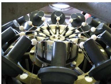
**Figure 4:** The top of the rosette of Niskin bottles, a water sampling apparatus. These caps snap shut, trapping the water inside as the sensor package descends through the water column. Each bottle can be closed electronically at a different depth, and captures 10 L of water, enough for a variety of chemical and biological assays.
